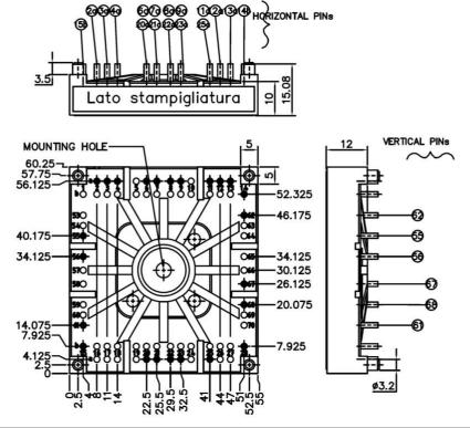
Case T 88 (Suggested hole diameter for the solder pins in the circuit board: 2mm. Suggested hole diameter for the mounting pins in the circuit board: 3,6mm)
